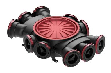
Distribution box with OneClick technology® is connected directly to the MHRV unit and used to supply fresh air into habitable rooms or extract used air from the "dirty" rooms.
