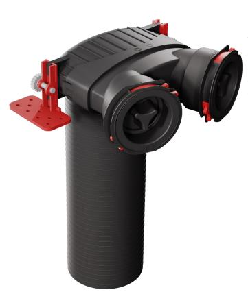
The plenum box with OneClick technology® allows the connection of up to 2 90mm ducts to a 125 mm supply / exhaust air diffuser. Factory-assembled, complete with a set of plugs and gaskets. Leave unused slots blanked. Constructed from high quality polyproylene.
