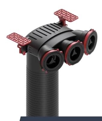
The plenum box with OneClick technology® allows the connection of up to 3 75mm ducts to a 125 mm supply / exhaust air diffuser. Factory-assembled, complete with a set of plugs and gaskets. Leave unused slots blanked. Constructed from high quality polyproylene.
